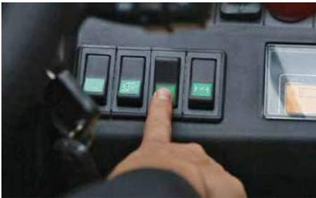
Full-floating hydraulic drive gear box has the function of switching between 2WD and 4WD, and can provide higher run speed and stronger climbing ability.
