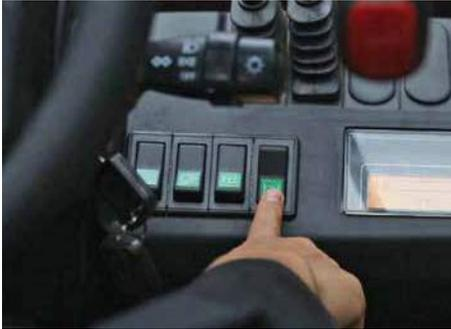
The differential is specifically designed for rough terrain and features manual differential lock providing ultimate traction during inclement weather conditions and rough operating surfaces, it differential lock prevents power loose when one wheel spins.
