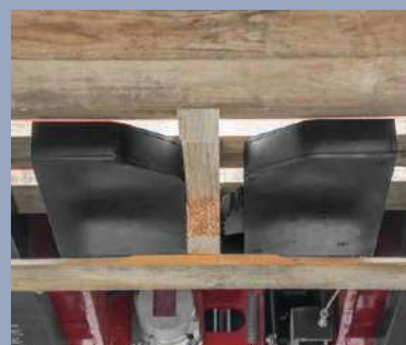
Manual-locking pallet clamp work on a wide range of pallets and accommodate pallet stringers ranging from 1" to 2" so operators can handle any pallet
